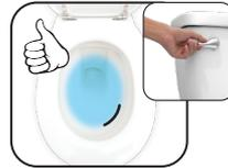
If the water level matches the line in the bowl and the fill valve is **STILL FILLING**, then the bowl water is **TOO HIGH**, proceed to Step 12D.
